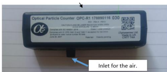
Figure 3: Optical particle counter (OPC) sensor to measure particulate matter. Produced by (and purchased from) Alphasense Ltd.
