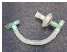
Figure 2: Breath sampling tube
