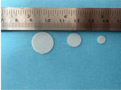
Fig. 1: example of 3D printed disks with different diameters.
