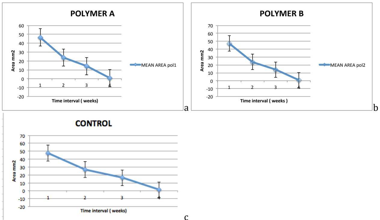
Figure 4 a,b,c: polymer A is poli-D-lactic acid with 10% of hydroxyapatite; polymer B is poli-  $\epsilon$  caprolactone with 20% of  $\beta$ - tricalcium phosphate; c is the control group.
