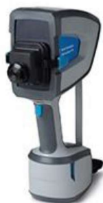
Figure 7.7: The Agilent 4300 ATR-FTIR spectrometer
