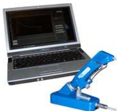
Figure 7.6: The Aquaflux TEWL machine
