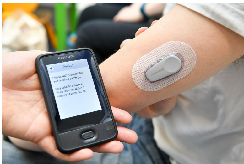
Figure 2: Dexcom G6 receiver paired with sensor patch with transmitter attached.
