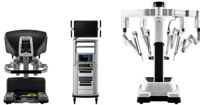
Figure 1: An example of a robotic platform (the Da Vinci Xi). From left to right, the devices shown are the surgeon console (where the surgeon sits to control the robot), the vision cart (the computer and brain of the platform), and the patient cart (the robot arms that hold and move the surgical instruments).
