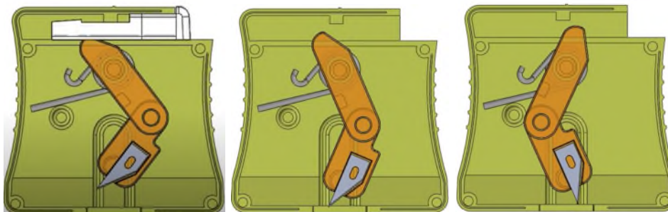
Figure 3: Schematic drawings showing from left to right the sweeping motion of the tri-bevel stainless steel blade after the blade is deployed.
