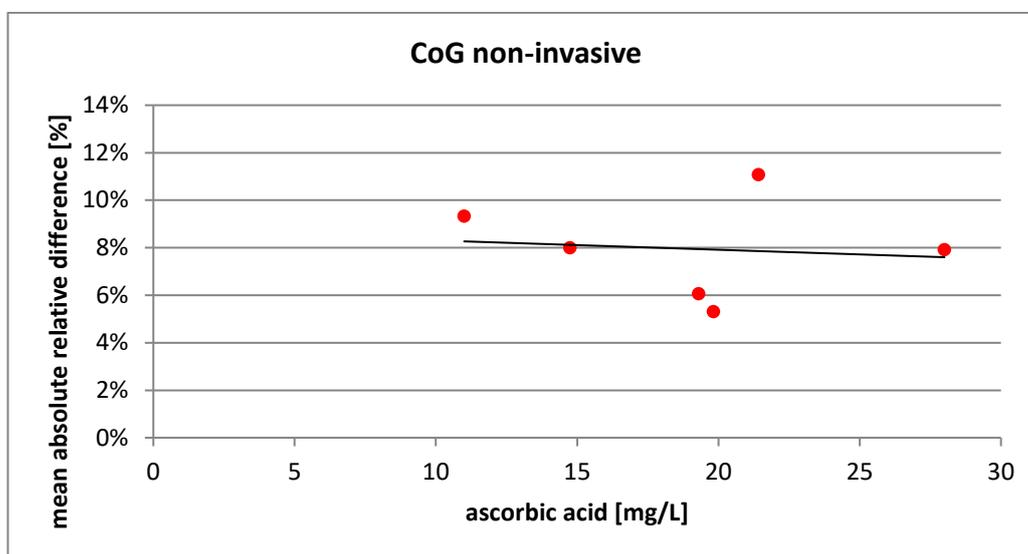
Figure 7.: MARD of the invasive CoG readings vs. YSI as a function of mean ascorbic acid concentrations (regression line:  $y=0.001*x-0.052$ ,  $r^2=0.283$ ).
