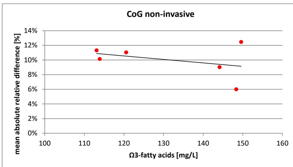
Figure 41.: MARD of the invasive CoG readings vs. YSI as a function of mean 3Ω-fatty acid concentrations (regression line:  $y=-0.001x+0.215$ ,  $r^2=-0.685$ ).
