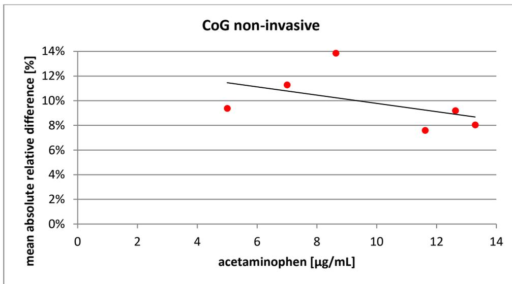
Figure 3.: Mean absolute relative difference of the invasive CoG readings vs. YSI as a function of mean acetaminophen concentration (regression line:  $y = -0.002 \cdot x + 0.086$ ,  $r^2 = 0.538$ ).
