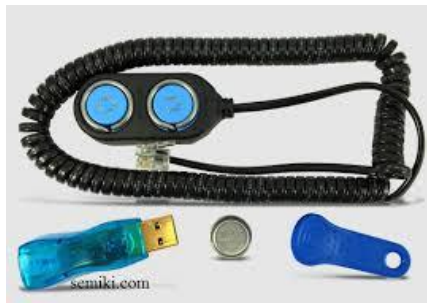
Figure 1: Hygrochron iButton temperature and relative humidity data logger used for indoor residential monitoring.
