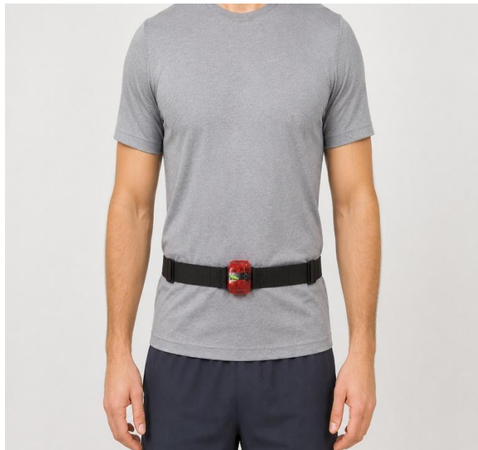
Figure 18. Waist-worn tri-axial accelerometer placement for activity monitoring.
