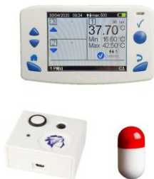
Figure 12. The e-Celsius receiver, activator and ingestible temperature capsule.
